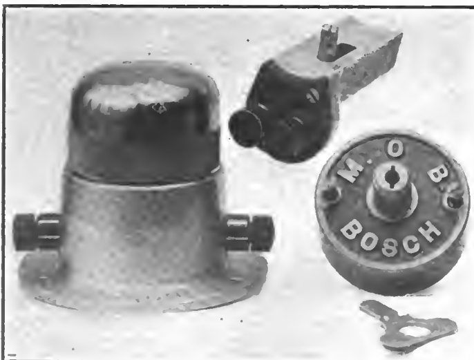
Fig. 3—Components of vibrating duplex system. The inclosed vibrating coil is at the left and the dash switch at the right
